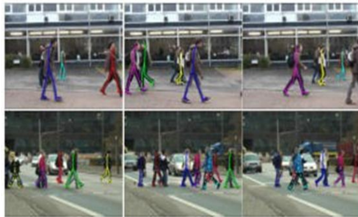
Figure 3: Examples of detection and tracking of specific persons in image sequences of crowded street scenes (Mykhalo, Stefan & Bernt, 2008)
