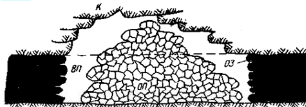
Pic. 3. Character of filling up degassed spaces as a result of a bending flexure of a roof rock
