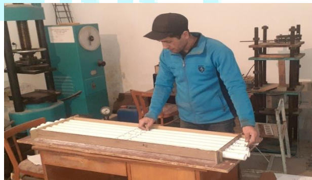
Fig.4. Hollow core formwork
