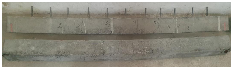
Rice. 9. Types of cracks in tested samples
