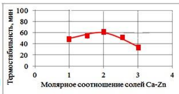
Picture 1. Influence of the molar ratio of calcium-zinc palmitates on the thermal stability of PVC at 160 °C: 1 – Ca salts: Zn salts = 1.25:0.75; 2 – Ca salts: Zn salts = 1.5:0.5; 3 - Ca salts: Zn salts = 1:1
