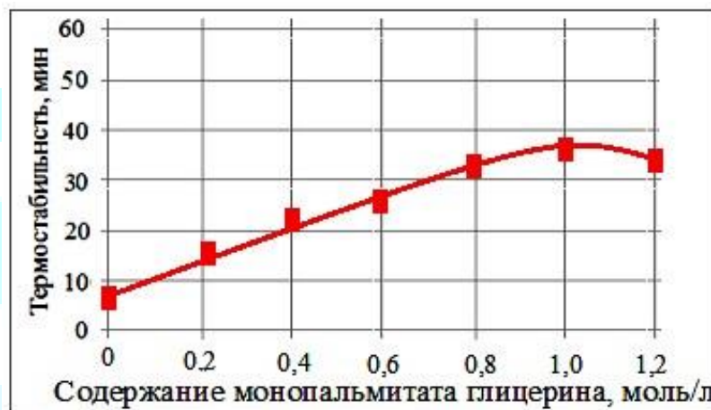
Picture 3. Dependence of thermal stability ( T = 190\text{ }^{\circ}\text{C} ) of PVC composition on the content of glycerol monopalmitate in the multifunctional stabilizer
