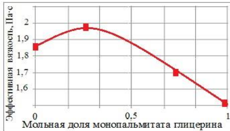
Picture 2. Dependence of the effective viscosity ( T = 180\text{ }^{\circ}\text{C} ) of PVC composition on the content of glycerol monopalmitate in the multifunctional stabilizer
