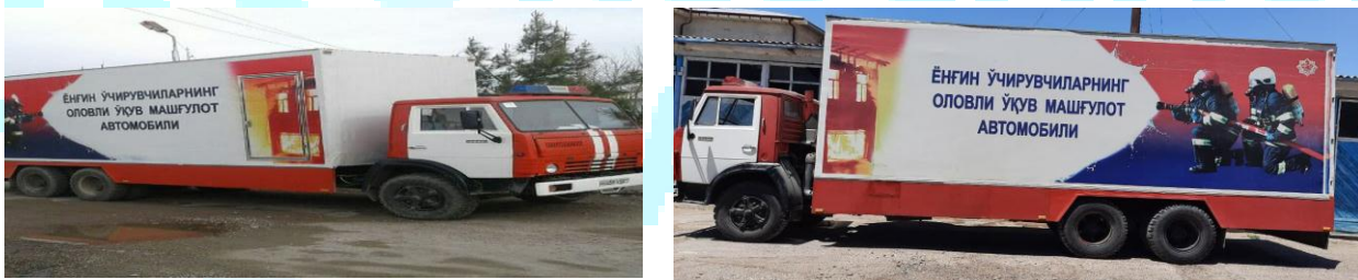
1-picture. On the proposed Kamaz-53229 chassis is a re-equipped "flame-training car".
