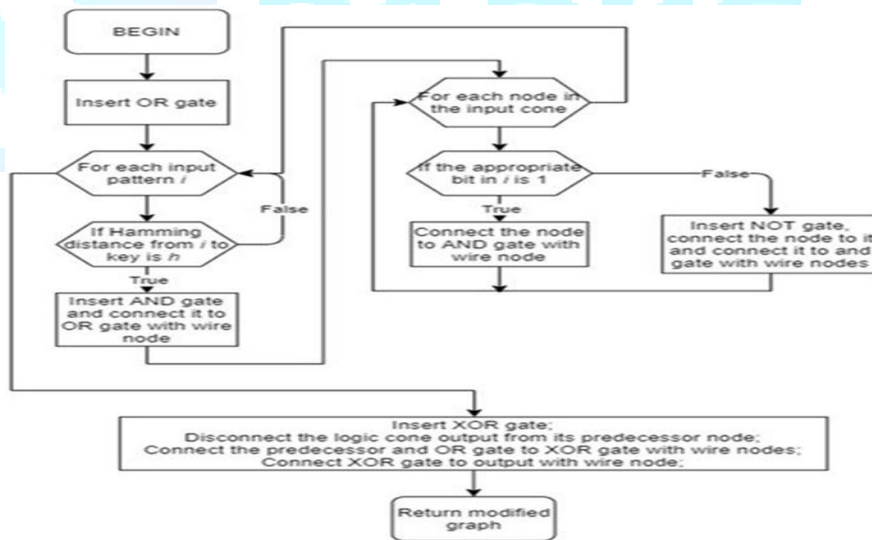
Figure 4: Flowchart for Inserting Logic Locking Gates
