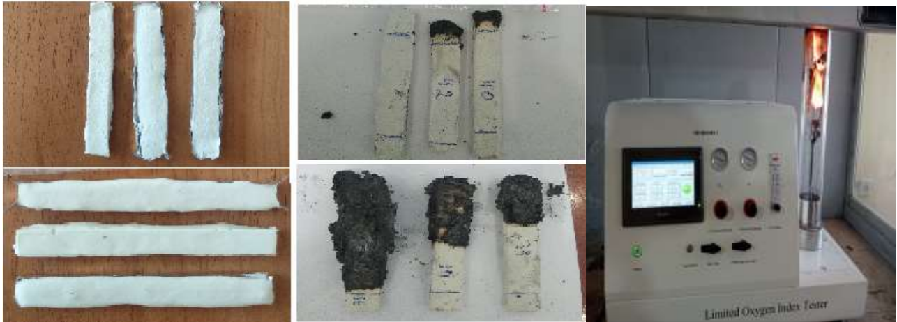
Figure 1. Laboratory procedures for researching the oxygen index of fire-resistant and heat-protective polymer composite coatings.
