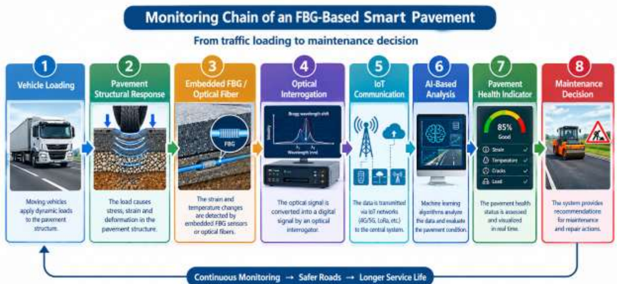
Figure 2. Conceptual monitoring chain from vehicle loading to maintenance decision.
