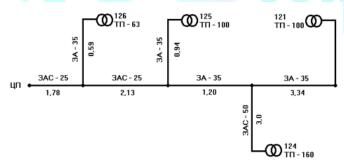
Design diagram of a 10 kV distribution network. The initial data for the calculation are the measured current at the head section of the feeder and the voltage on the buses 0.38 - 6 - 10 kV on operating days, as well as the rewards of all or part of the transformer substations [4].
